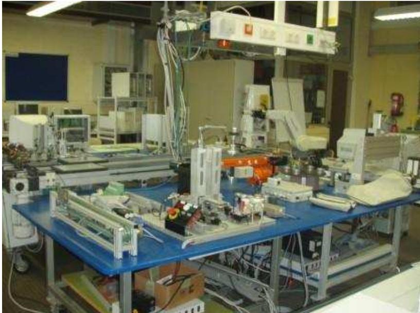
It is about a mechatronic production system where workpieces are transported on a band-conveyor to several stations (material detection and drill).
